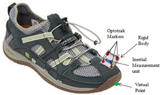
Fig. 2. Rigid body and inertial sensor arrangement on the shoe
