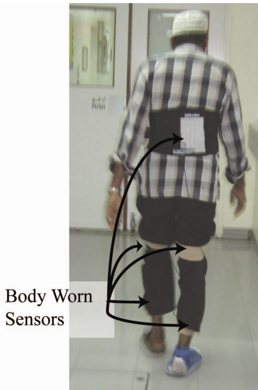
Fig 1. LegSys™. A wearable sensor technology for extracting spatio-temporal parameters of gait outside of a gait laboratory, over different footwear condition, walking surfaces, and in the environment where may better mimic true patient's living environment.
