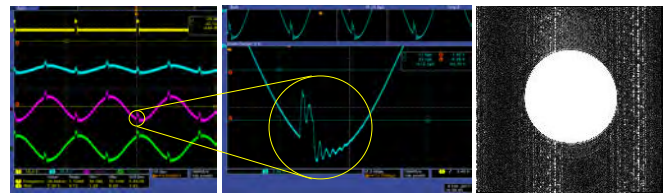
Fig. 3. Driving waveforms from off the shelf nanomotion driver (left). Closeup view of a high frequency artifact (center). Scanner image taken of a motor being operated by this driver [8] showing a high degree of distortion and noise (right).
