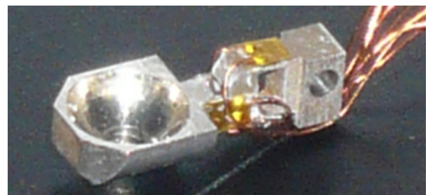
Fig.5. Manufactured clip and fit strain gages
