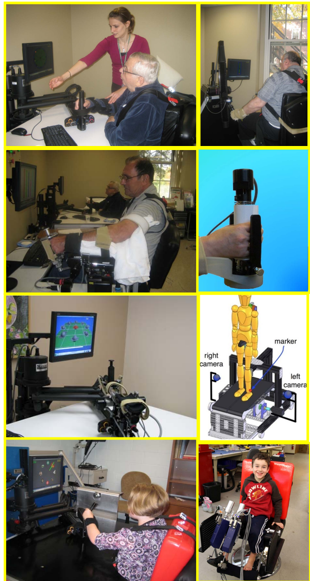
Fig.2. MIT Gym of Robots [7, 11-17]. Top row on the left shows the MIT-Manus to promote neurorecovery of the injured brain and control of the shoulder-and-elbow and on the right the anti-gravity to promote training of the shoulder against gravity. On the 2 nd row on the left we show the wrist robot which affords training of the 3 degrees of freedom of the wrist and forearm and at the right, the hand module for grasp and release. The 3 rd row on the left shows the combination of shoulder-and-elbow robot with the wrist module mounted at the tip of first affording training for both transport of arm and object manipulation. On the right, the sketch of the alpha-prototype of the MIT-Skywalker for gait training. On the bottom row, we show pediatric populations working with the MIT-Manus and our pediatric anklebot that afford training in dorsi/plantarflexion and inversion/eversion.
