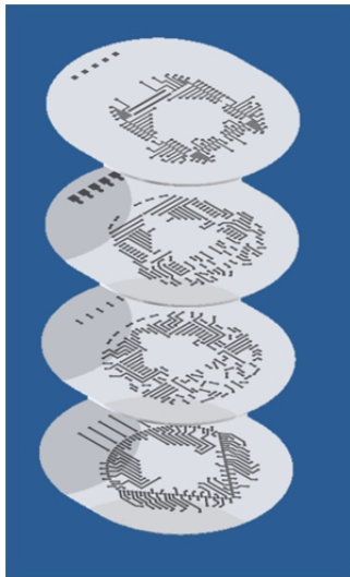
Fig. 2. Exploded view of the four layer substrate showing the routing of the Pt tracks from the chip side to the electrode side.
