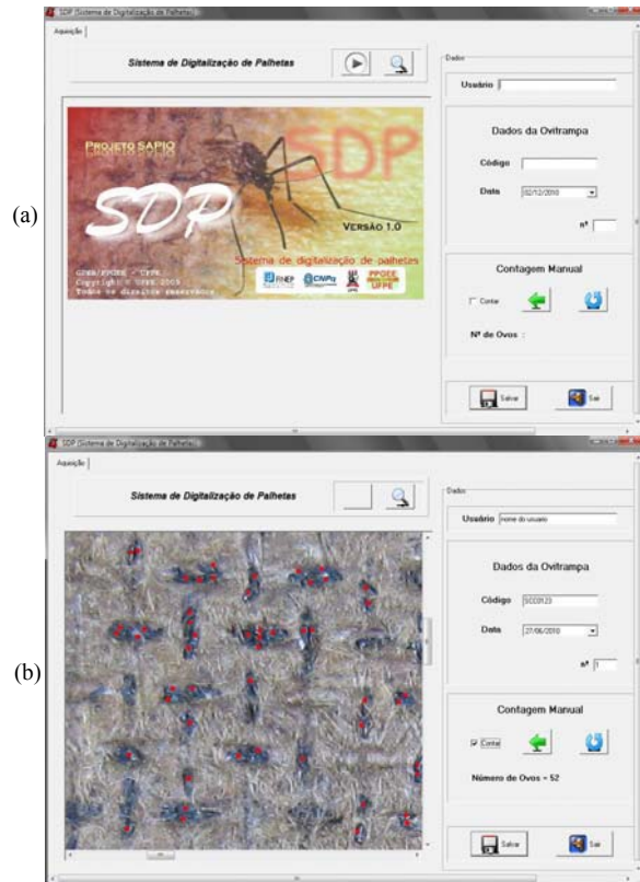
Fig. 4. Human-Machine Interface, (a) entry screen, (b) after image acquisition, with manual counting computer-assisted, where the eggs are marked with red dots and (c) eggs marked with red dots to score computer-assisted.
