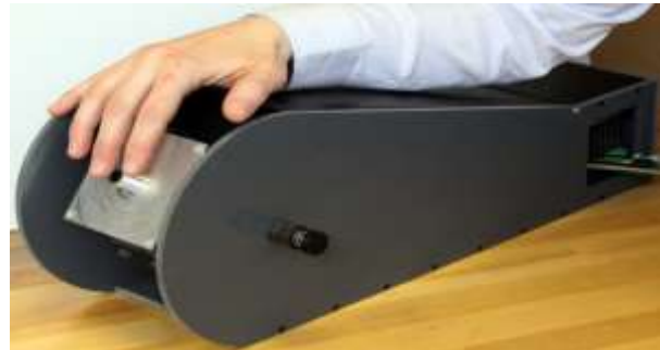
Fig. 2. The Vibrotactile Threshold Evaluator for Workplace Screening (VTEW) with the cover removed to show the surround and probe [8].
