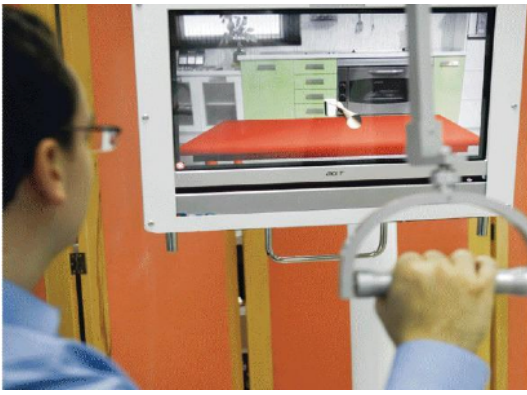
Fig. 2. Virtual reality software of the Pneumatic Rehabilitation Robot
