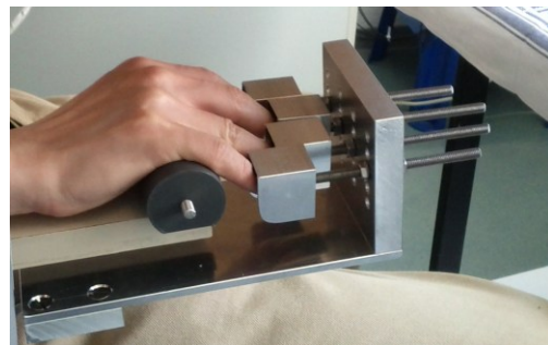
Fig 2. A mechanical structure restricted the range of finger movements for the hand fixed block. The extension of each finger was controlled by this.
