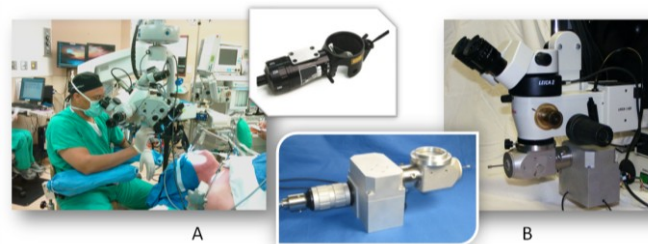
Fig. 1. Laser aiming systems: (A) traditional phonomicrosurgery setup: mechanical micromanipulator (UniMax® Micromanipulator by Laser Engineering, Nashville, TN, USA) coupled with a surgical microscope (picture copied from [4]); (B) IIT's system: computer-controlled motorized micromanipulator coupled with surgical microscope.
