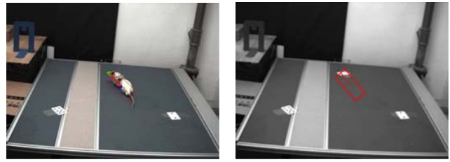
Fig. 1. The video with the position and orientation is computed and marked colored (left); the processed video with which the body of rat-robot is replaced by a rectangle, and a red line points to the head's direction.
