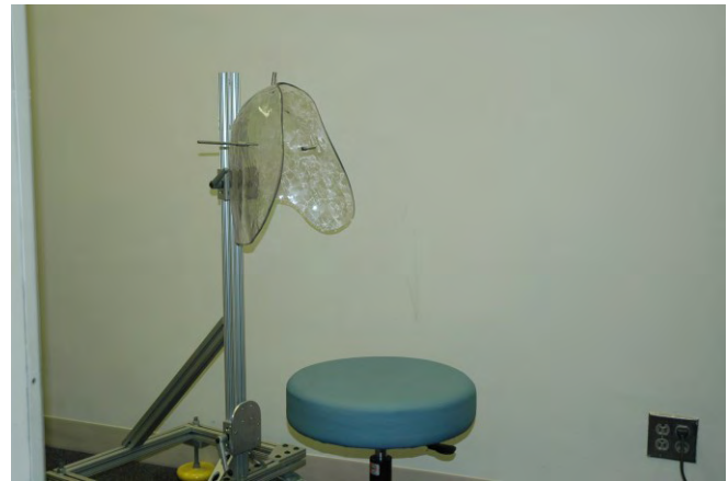
Figure 2: Test Setup to Measure Shoulder Range of Motion and Force
