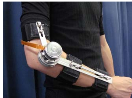
Fig. 1 Exoskeletal robot for ET patient [4] [5] whose concept is not only mechanically suppress tremors, but can also voluntarily movement.
