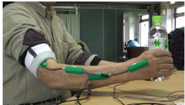
Fig. 2 Measurement of surface EMG signal and elbow joint angle. The subject performed elbow flexional movement while holding a bottle filled with water (mass 550(g)).
