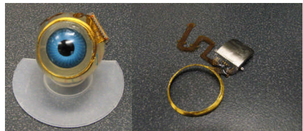
Fig. 2. Second-generation hermetically-packaged 16-channel Boston retinal prosthesis.
