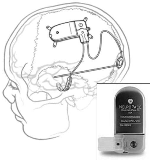
Fig. 1. Typical NeuroPace RNS ® System implant configuration is shown in schematic view, with inset showing the implantable neurostimulator. Up to two leads may be connected to the neurostimulator; either may be a depth lead or cortical strip lead with electrodes placed at or near the seizure focus.
