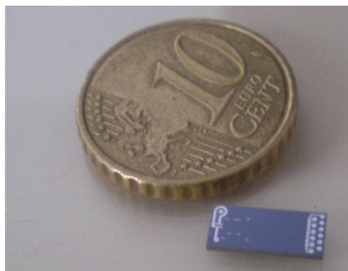
Fig. 2. Photograph of a chip accommodating 10 monolithically integrated FR-MZIs.
