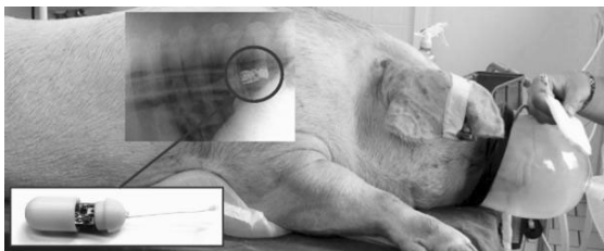
Fig. 3 Animal experiment. The transmitter was placed near the heart (circle). The transmitter and the power supply were put into the capsule. To get the real position in the esophagus, an X-ray photograph was taken. This picture is a photo montage of the X-ray and the real photograph.
