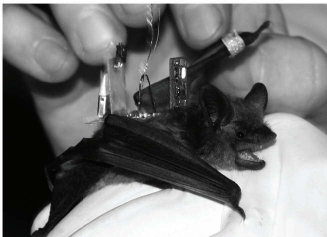
Fig. 1. A bat equipped with a wireless ultrasound microphone and prepared to fly while tethered to a zip line.
