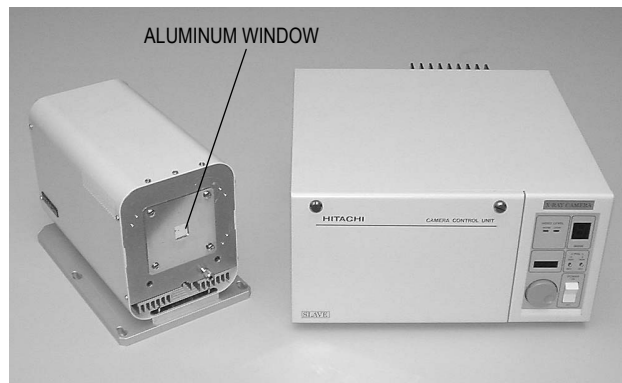
Fig. 2 Photograph of the X-ray SATICON camera system comprising a camera head (left) and a camera control unit (right).
