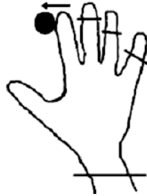
Fig. 1 – Schematic representation of the technique used to capture a participant’s isometric force response. The horizontal lines drawn through the wrist and fingers imply that these areas were secured to the test platform to prevent accidental movements. The index finger applies an abductive force to a force detector (black circular object) in the direction shown by the arrow in the figure.
