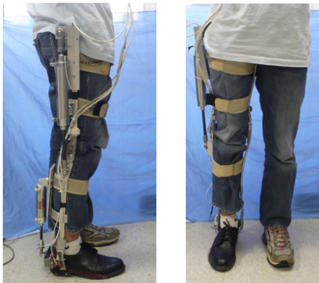
Fig. 1. The lower-limb orthosis fitted to a healthy subject.
