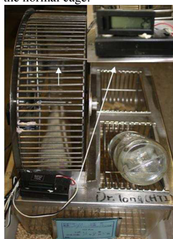
Fig. 2. the wheel training system: a switch counts and records the number of revolutions.
