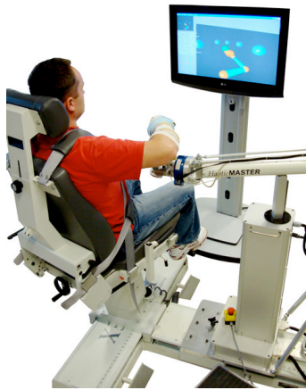
Figure 1. Set-up for assessment of total reaching work area with the ACT 3D .
