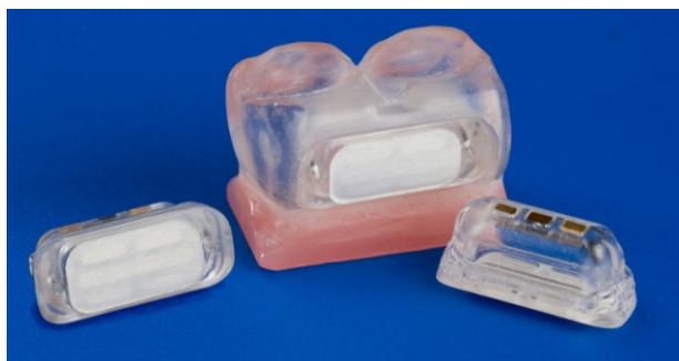
Fig. 4. Prototype of the Cartridge and the partial removable prosthesis.
