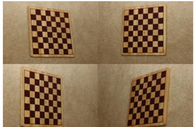
Fig. 2. Images of checkerboard for camera calibration.
