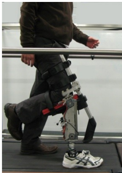
Fig. 3. Able body subject using kneeling socket adaptor to test active knee prosthesis on a treadmill.
