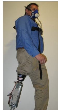
Fig. 4 Unilateral above-knee amputee wearing portable K4b2 telemetric system equipment for metabolic cost assessment.
