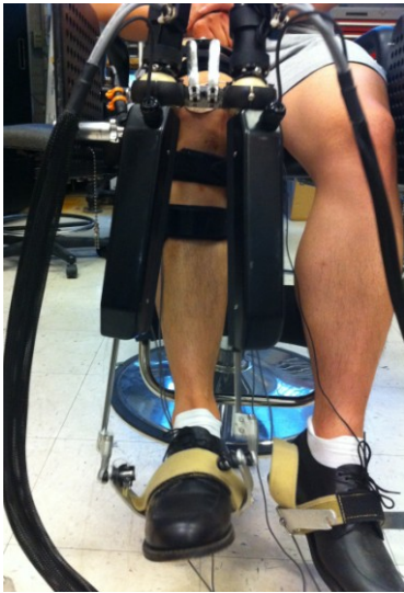
Fig. 1. Subject wearing Anklebot in a seated condition
