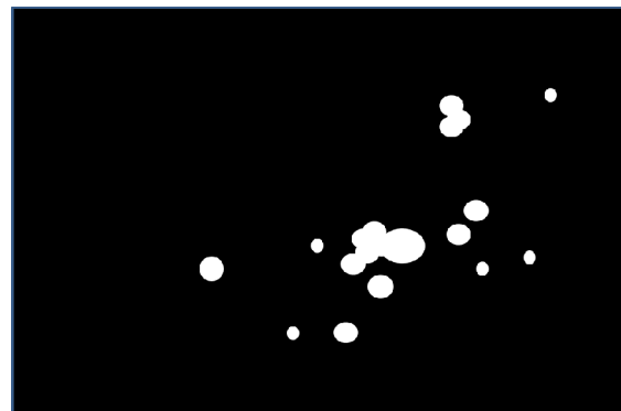
Fig. 4. Candidate ROIs for retrieving keypoints with h=0.03 in SIFT algorithm
