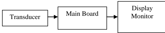
Figure 1: Basic components of an ultrasound machine
