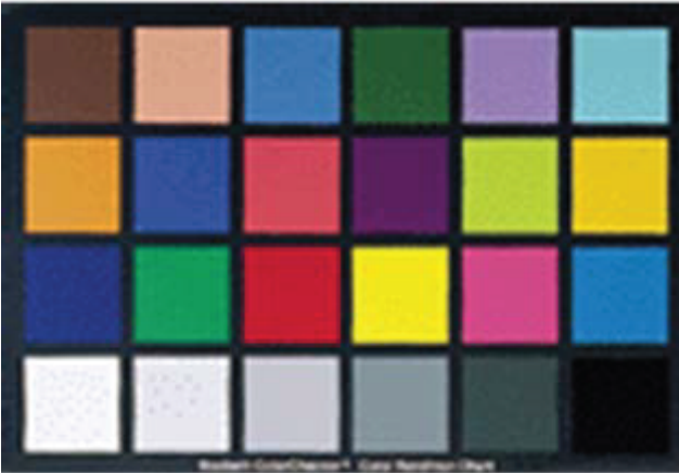
Fig. 1. The testing targets of the color palette with known color distribution from the Edmund Industrial Optics Company [15]
