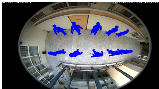
Fig. 6. The 3D model of a standing man, rendering the 3D human models through the fisheye camera model.
