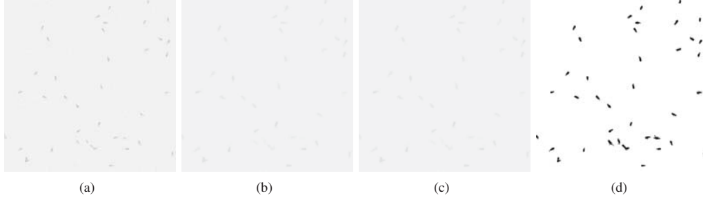
Fig. 3. The preprocessed microscopy image based on mathematical morphological. (a) Original image. (b) Image after MM operators. (c) Opening-closing by morphological reconstruction. (d) Regional maxima of morphological reconstruction.
