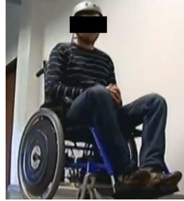
Fig. 11. Functional test of wheelchair controlled by cervical movements
