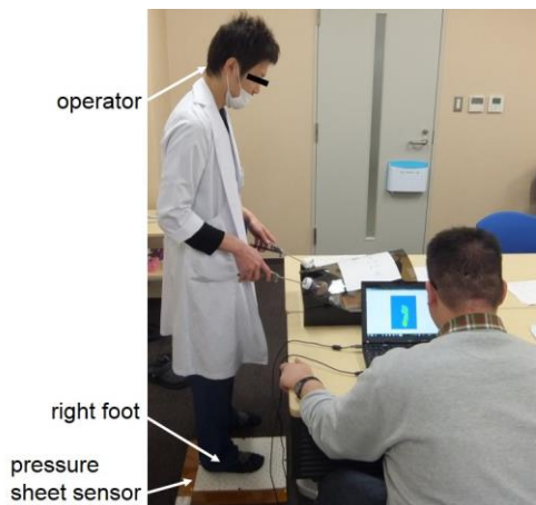
Figure 2. Experimental setup for measuring the temporal changes in the center of gravity of the foot, together with the applied force using a pressure sensor sheet.
