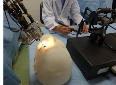
Fig. 7 Master-slave robotic system for eye surgery
