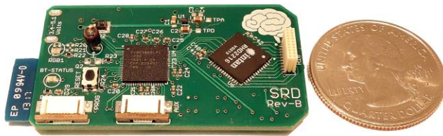
Figure 2. Photo of our current SRD PCB (27 mm x 48 mm) next to a US quarter dollar for reference.
