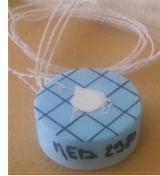
Figure 2. A thermal canal made with silicone thermal semiconductor (white core) insulated with polystyrene (blue envelop).
