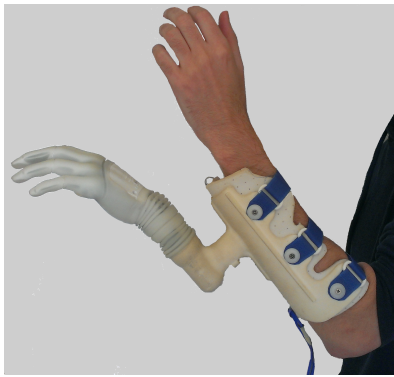
Fig. 1. A subject wearing the Michelangelo prosthesis with the able-bodied adapter.
