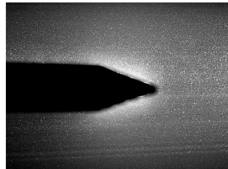
Fig. 3. Typical image for DIC with \text{Al}_2\text{O}_3 particles scattering light around a blade with a tip angle of 40^\circ
