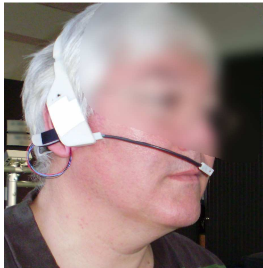
Fig. 1: Multi-sensor headset for robust heart rate and ventilatory rate measurement
