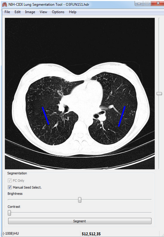
Fig. 1. Manual seed selection in CIDI-Lung-Seg. Single-stroke painted line (shown in blue ) are used as seeds for left and right lungs.
