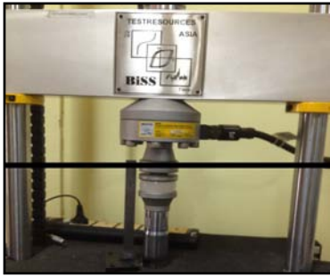
Figure 1: Universal compression testing machine with one of the phantoms positioned between the compression plates.
