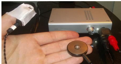
Figure 2: The Schiit Magni headphone amplifier receives input from a computer’s audio card. It provides stereo out which is split between two RCA connectors. Each C-2 tactor (shown here in the palm and on thumb) receive an analog audio signal which is converted to a vibration.
