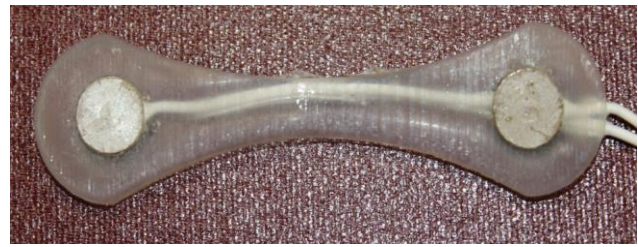
Fig. 3. Sintered Ag/AgCl electrodes cast in silicone elastomer
