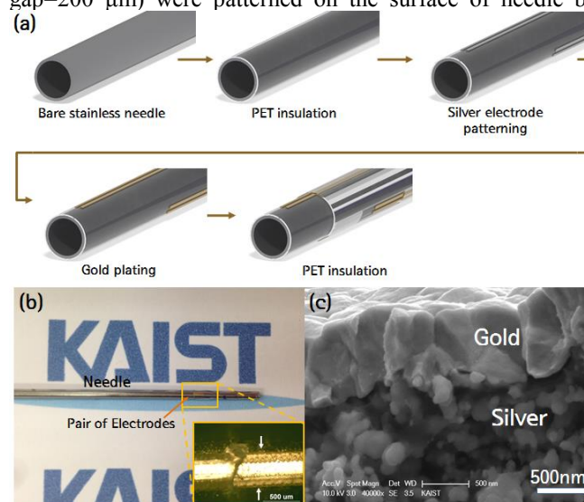
Figure 1. (a) Schematic diagram of fabrication process and (b) photograph of the impedance sensing needle; (c) The cross-sectional image of the gold-plated electrode.
