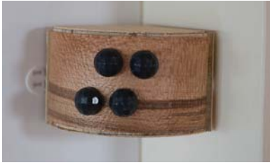
Fig. 1. Installed PIR sensor, constructed using four PIR transducer elements to cover blinds zones.
