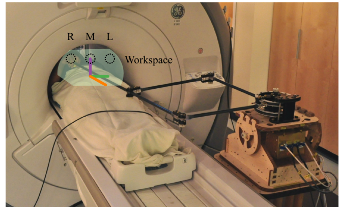
Fig. 1. Motor Neuroimaging with Haptic fMRI. The experiment involved planning and executing goal-directed reaches to three distinct spatial locations (left, L; middle, M; right, R) that spanned the MRI workspace. A three degree-of-freedom fMRI-compatible haptic interface, HFI, monitored hand motions. A real-time virtual simulation provided visual feedback on a screen behind the scanner.
