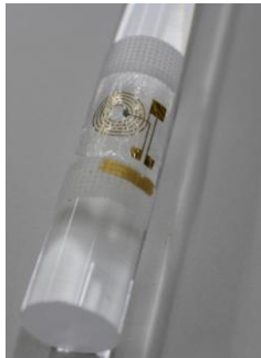
Figure 3. Experimental methods for evaluating the pressure-sensitivity and flexibility. (a) Circuit characteristics were measured using an LCR meter with an external pressure applied on the capacitor. (b) The device is contoured to conform to a rod, showing that the device can be attached on a stent graft. (c) The device was immersed in agar for MRI acquisition.
