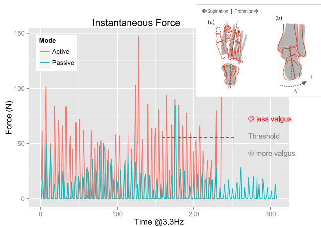
Figure 2. Instantaneous force sensor reading at outer midsole point of an untrained subject. Passive: valgus walk. Active: the patient is instructed to walk while actively correcting valgus (calcaneal inversion) posture by using foot muscles. A force threshold can be set to discriminate healthy from unhealthy postures. (a) Plantar view. (b) \Delta is calcaneal inversion in degrees. Top right adapted from [6].
